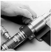
Refer to the label on the vortex tube to determine the shaft position for warm and cool air.
