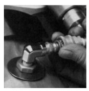
Be sure the quick-disconnect fitting and plug snap into place. Gently tug on the connection to ensure it's tight. Cool (or warm) air should begin to flow into the protective suit immediately. Enter the work area.
